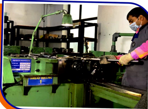
Thread Rolling Machine 40 Ton Capacity
